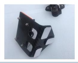
**Step 3** – Decide where you want to fit the compass mounting and align it accurately. Put a few pencil marks around the corners. The mounting is best fitted just aft of the control line blocks under the vang assembly.
