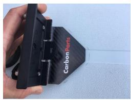
Step 6 –Press very firmly at the front and at the rear where the compass mountings are to ensure that the adhesive pads are pressed onto the deck. Keep pressing for a minute if possible. DO NOT try and remove the mounting yet.
