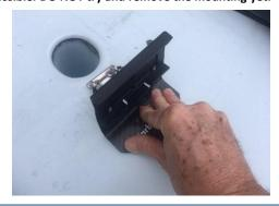
**Step 7** – Leave the compass mounting in position for as long as possible. DO NOT attempt to remove the compass mounting for at least one hour, or you may pull the mountings from the deck.
