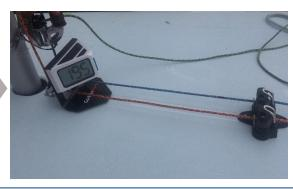
If your mountings don't successfully stick to the deck it is probably because the deck was not absolutely dry. If you have any problems, or need replacement mounting pads please contact us at info@carbonpartsgermany.de Garbon Parts
